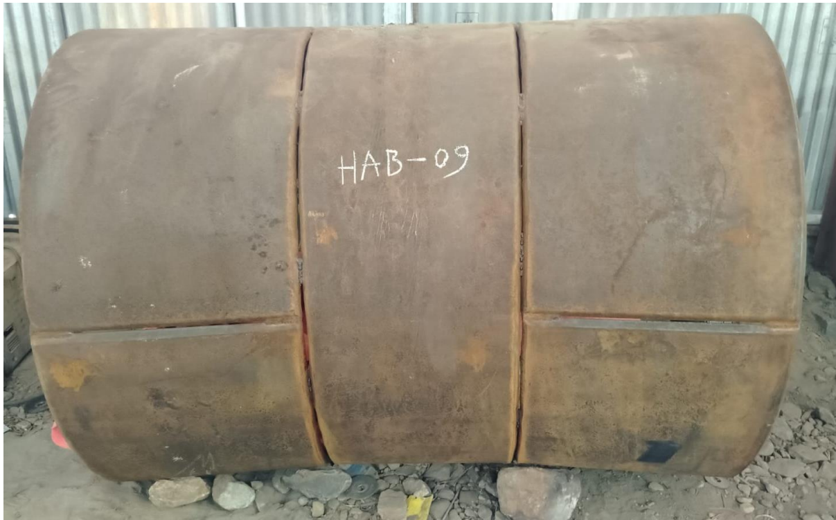
Figure 16: Anchor block 9 bend pipe in site workshop
